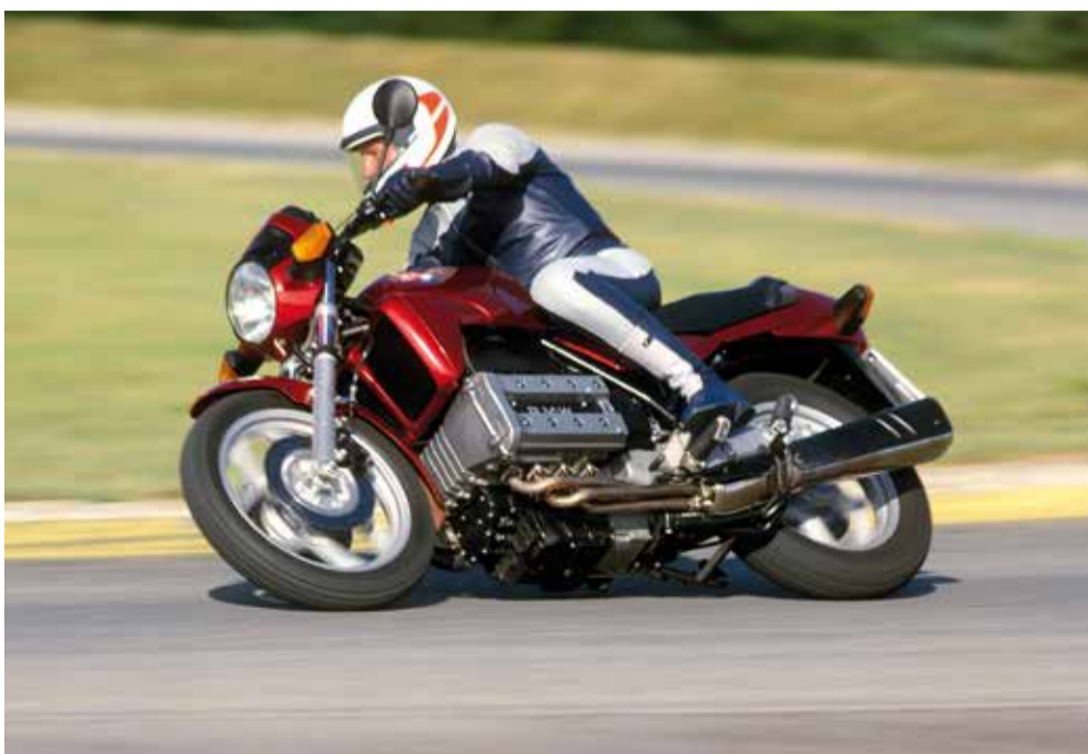
The BMW K 100 was introduced in 1983 and it was completely different from anything BMW had ever done until then. It had a horizontally placed in-line four cylinder engine that was liquid cooled and produced 90 hp. Strong, fast and reliable, it proved to be quite successful.
