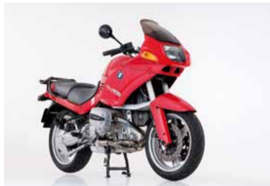
The R 1100 RS started a new generation of boxer models, being designed from scratch. The Telelever front suspension provided excellent stability without compromising handling and the 1,085 cc engine was fuelled by electronic injection, a premiere for BMW boxers.
