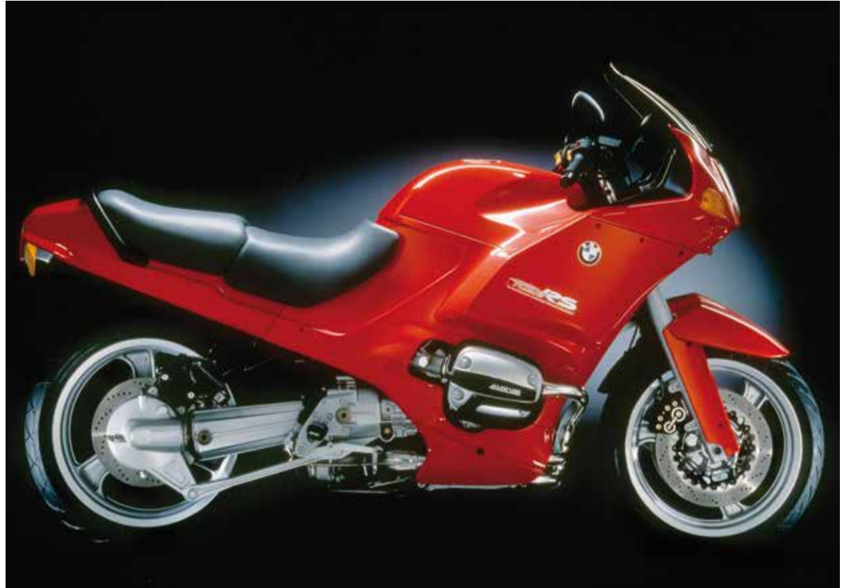
The R 1100 RS started a new generation of boxer models, being designed from scratch. The Telelever front suspension provided excellent stability without compromising handling and the 1,085 cc engine was fuelled by electronic injection, a premiere for BMW boxers.
