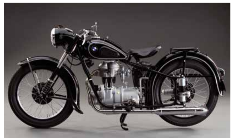
The BMW R 25 evolved from the R 24 in 1950, with a steel tube frame and dampened rear suspension. In two years, over 25,000 units have been produced.
