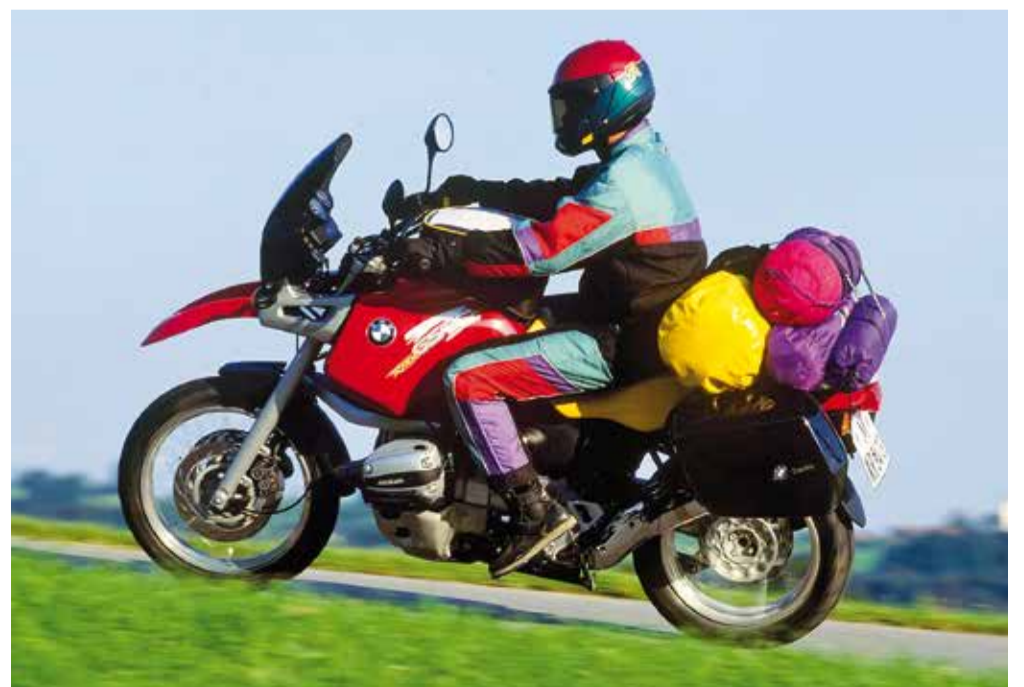
The R 1100 GS, launched in 1994, was the first BMW GS from the '90s and it had a fuel injected engine, Telelever front and Paralever rear suspension. It instantly became the vehicle of choice for globetrotters across the world.
