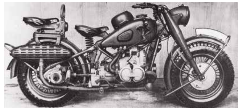
The BMW R 75 was the warhorse of the German army. Strong and reliable, it had amazing off-road abilities, thanks to its transfer box.
