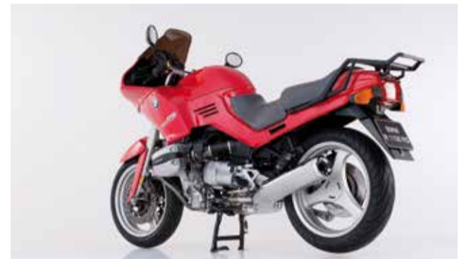
The R 1100 RS started a new generation of boxer models, being designed from scratch. The Telelever front suspension provided excellent stability without compromising handling and the 1,085 cc engine was fuelled by electronic injection, a premiere for BMW boxers.
